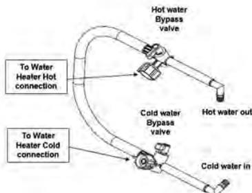
**Two Valve Water Heater Bypass**
