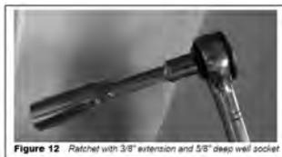
Figure 12 Ratchet with 3/8 inch extension and 5/8 inch deep well socket
