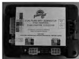
Fig.1 Slideout Controller
