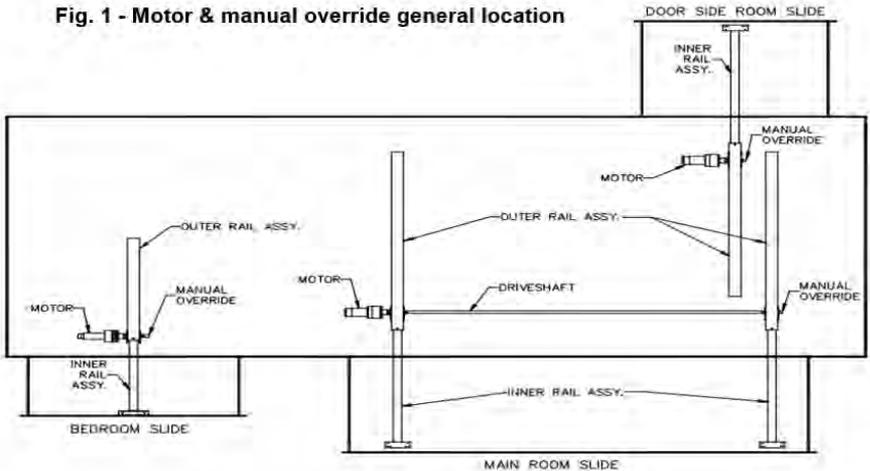
8. The room is now free to move. Using either a 5/8" or 3/4" wrench or socket, crank the room either in or out completely. If the slideout system is supplied with a gearbox override (optional), use the crank handle to move the room.
