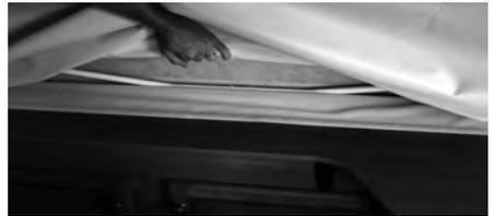
If the tent or hinge cover is not clear of the door edges, the door will not close and seal tightly, and/or damage to the bulb seal may occur.
