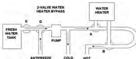
**NORMAL** – VALVE HANDLES A & B POINT TOWARD THE WATER HEATER.
