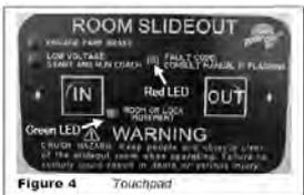
8. Release the OUT button when the room is fully extended or the IN button when fully retracted, and stops moving.
